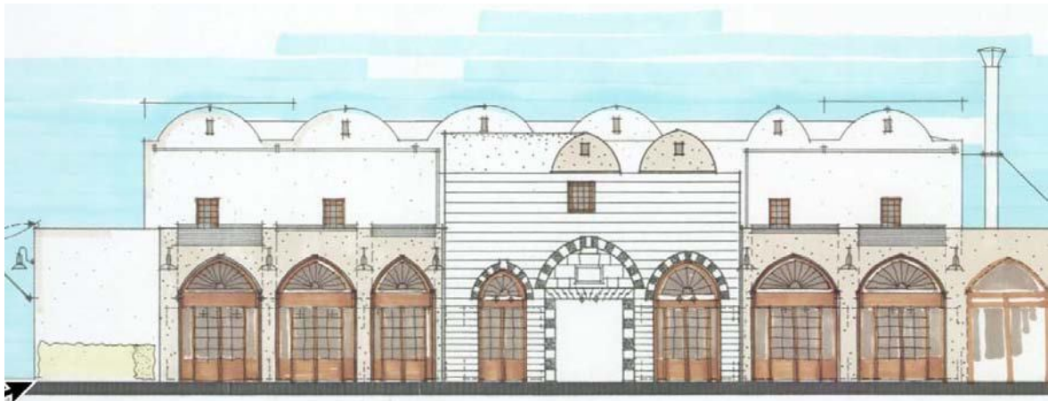
Khan el-Masriyyine. Facade towards east. Note the ablaq decorations on the main entry of the khan, now being part of souk el-Basarkan.
